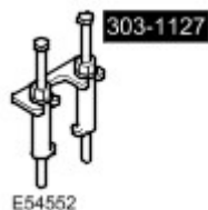
Remover - Fuel Injector 303-1127
